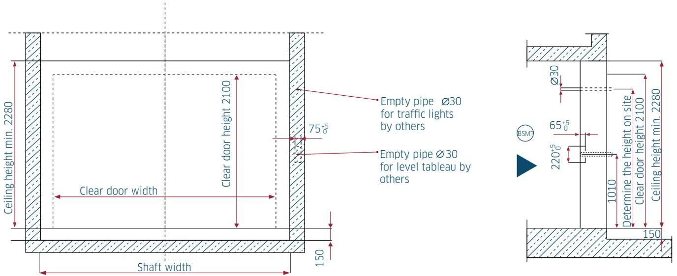
Door / edge protection passable with axle load over the entire opening width, by others!
