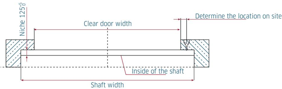
Door threshold / edge protection passable with axle load over the entire opening width, by others!
